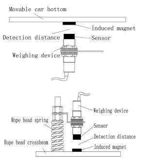
magnet is adsorbed at the crossbeam under the rope head with the logo side facing upward. The weighing device should be fixed on the rope head spring by the support frame, and the center of the magnet should align the center of sensor on weighing device, and the end surface of the weighing device should be parallel to magnet end surface. Adjust this device up and down slowly, keep the weighing device just at the point that the LED turns bright from dark, and fasten it.
